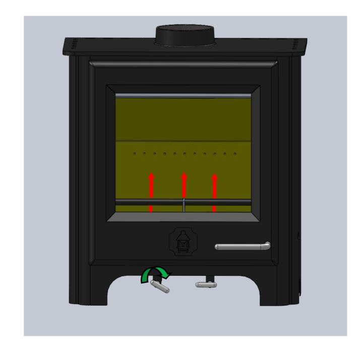
Large air settings can produce damaging temperatures to the stove and push wasted heat up the flue. This will be apparent if you look at the speed, colour and ferocity of the fire.
