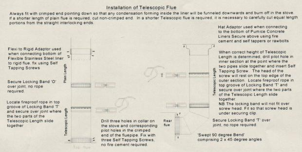
Locking band 'T' used when securing Telescopic Length to fluepipe below and to seal joint where interlocking sections slide together. All other joints between sections of fluepipe are secured with Locking Band 'O'.
