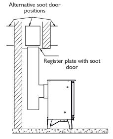
Fig. 7 Horizontal Register Plate With Top Flue Connection
